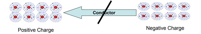
Materials that do not conduct electricity are called **Insulators**. Insulators do not allow electrons to flow through them
