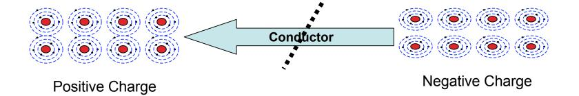
Some materials allow electrons to flow very slowly - they do not stop the flow, but they do **Resist** the flow A bit like you riding a bicycle with the breaks rubbing on the wheel - You can go along the road but you can't go as fast and there is one other effect - the break shoes will get hot - resistors produce **heat**.
